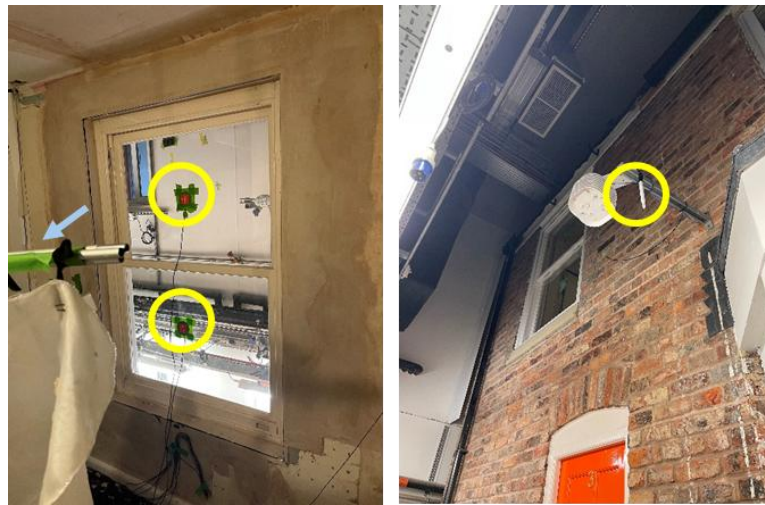
Figure 1 – Single glazed test window. Internal (left). Centre pane heat flux plates circled. The heat shield and internal temperature sensor (located out of frame) are denoted by the blue arrow. External (right). Temperature sensor circled.
